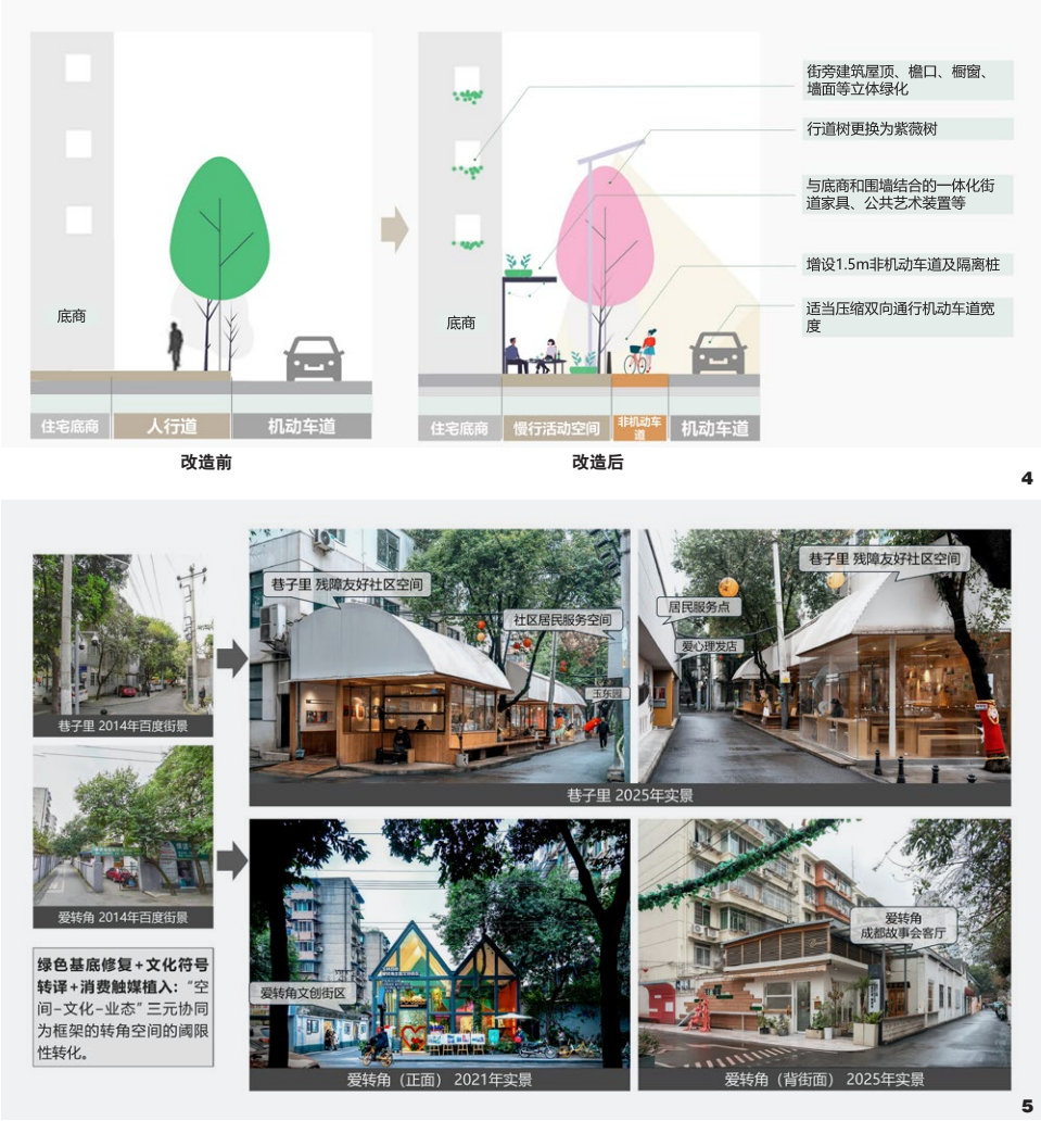
图4 玉林东路改造前后剖面示意图对比 Fig. 4 Comparison of cross-sectional schematic diagrams of Yulin East Road before and after renovation
