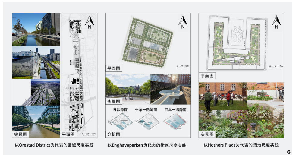
图5 结合蓝绿基础设施的雨洪管理措施 Fig. 5 Stormwater management measures coupled with blue-green infrastructure
