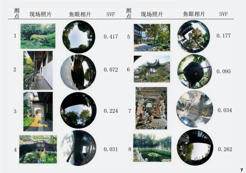
图5 测试点风速 Fig. 5 Wind speed at test point 图6 测试点生理等效温度 Fig. 6 Physiological equivalent temperature of test point 图7 测试点1-8现状及天空视域因子 Fig. 7 Status and sky view factor of test points 1-8
