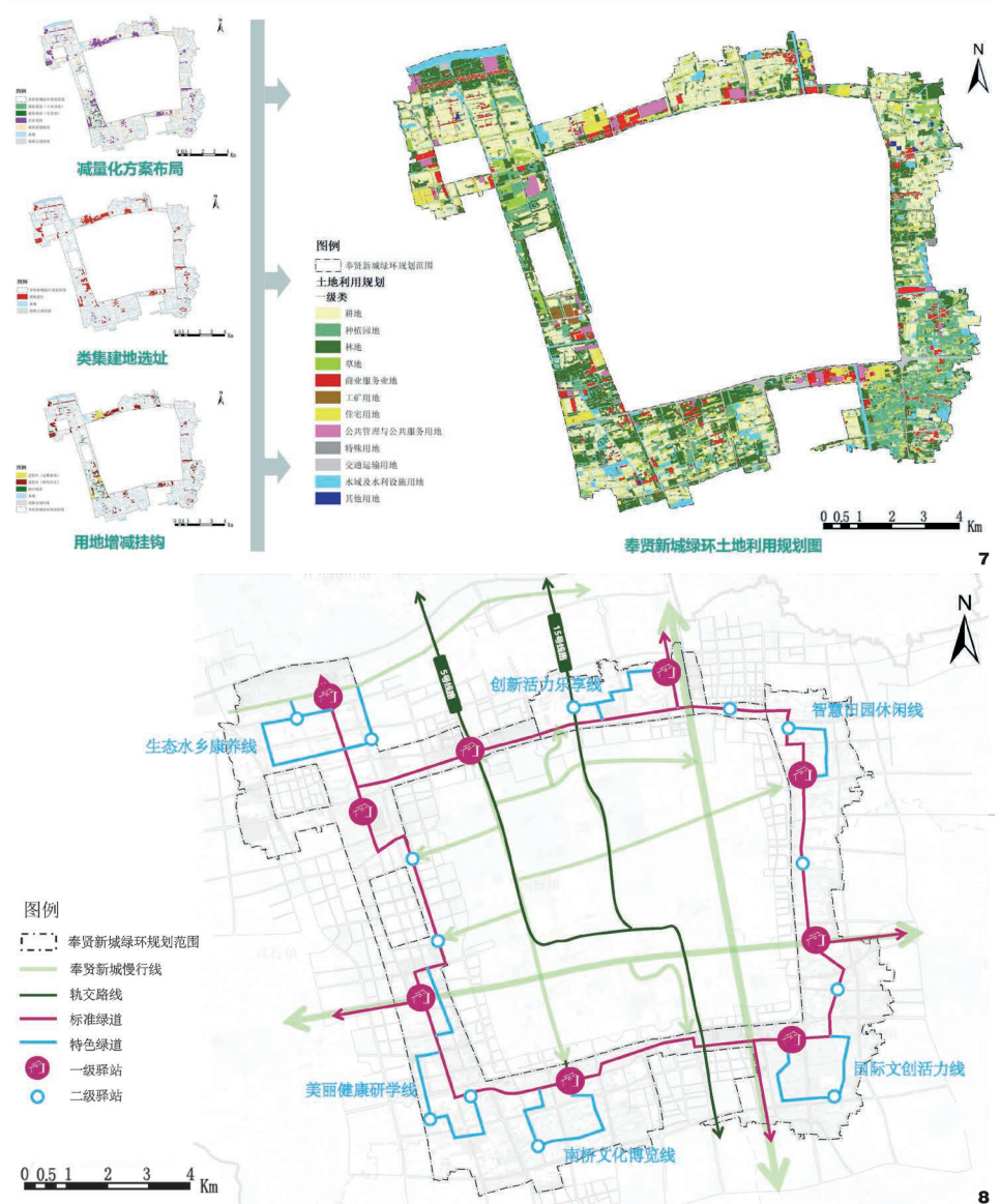
图7 奉贤绿环土地优化利用方案 Fig. 7 The optimal utilization scheme of Fengxian green belt land resources
